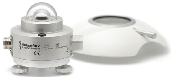
**Figure 4** SR20 with its sun screen removed
